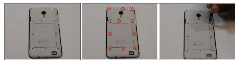
• Using one of the small Phillips screwdriver bits provided unscrew the 11 screws present on the protective plastic plate under the device case.
